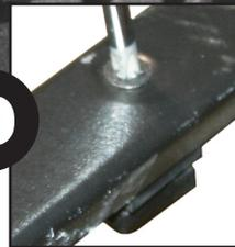
**4.** With the rails in place. Tighten down the screws in three locations on the rail with phillips screwdriver.
