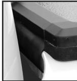
Place dust seal between cab and truck bed.
